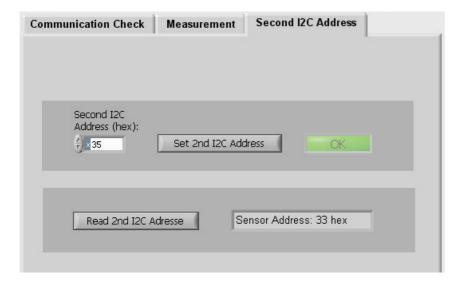
Figure 6: View on submenu "Second I2C Address"
