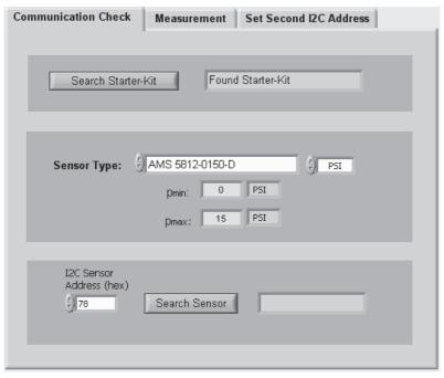
Figure 3: Overview of submenu "Communication Check"
