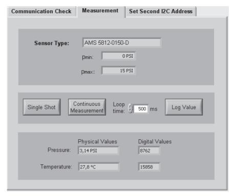
Figure 5: View on submenu "Measurement".
