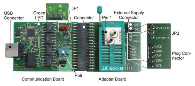
Figure 1: USB Starter Kit AMS 5812 with connected sensor.
