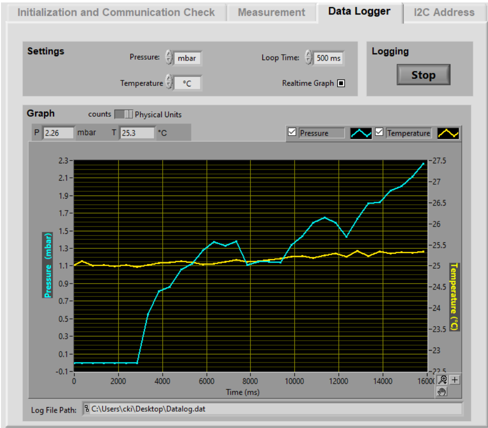
Figure 5: Data Logger Register: The button in the Logging field of the register starts and stops a continuous data measurement. The pressure and temperature readings are displayed graphically and stored in a data file.
