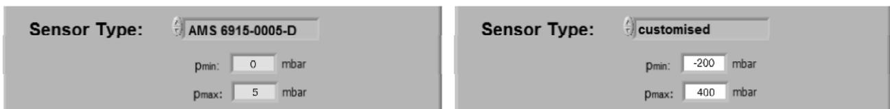
**Figure 5:** Selection of the used AMS 6915 sensor type.
