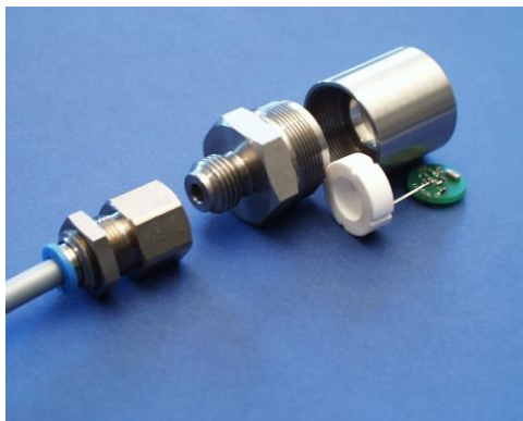
Figure 3: Complete prototype assembly with a pressure connection
