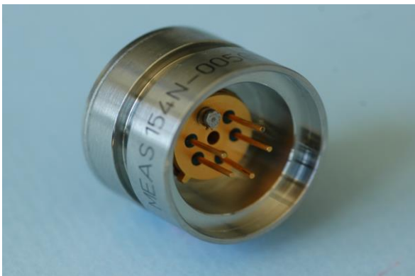
Figure 5: view of an absolute pressure sensor with an oil seal (reverse)
